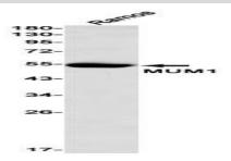
Western blot detection of MUM1 in Ramos cell lysates using MUM1 antibody(1:1000 diluted).
