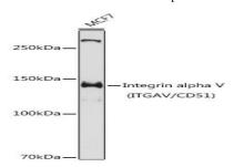
Western blot analysis of extracts of MCF7 cells, using Integrin alpha V antibody at 1:3000 dilution.<br/>
