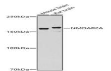
Western blot analysis of extracts of various cell lines, using NMDAR2A antibody at 1:1000 dilution.<br/>Secondary antibody: HRP Goat Anti-Rabbit IgG at 1:10000 dilution.<br/>br/>Lysates/proteins: 25ug per lane.<br/>br/>Blocking buffer: 3% nonfat dry milk in TBST.<br/>br/>Detection: ECL Basic Kit .<br/>br/>Exposure time: 180s.
