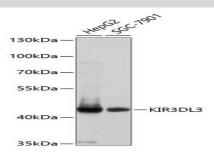
Western blot analysis of extracts of various cell lines, using KIR3DL3 antibody at 1:1000 dilution.<br/>Secondary antibody: HRP Goat Anti-Rabbit IgG at 1:10000 dilution.<br/>br/>Lysates/proteins: 25ug per lane.<br/>br/>Blocking buffer: 3% nonfat dry milk in TBST.<br/>Detection: ECL Basic Kit.<br/>br/>Exposure time: 15s.
