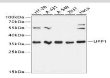
Western blot analysis of extracts of various cell lines, using UPP1 Antibody at 1:3000 dilution.<br/>Secondary antibody: HRP Goat Anti-Rabbit IgG at 1:10000 dilution.<br/>br/>Lysates/proteins: 25ug per lane.<br/>br/>Blocking buffer: 3% nonfat dry milk in TBST.<br/>Detection: ECL Basic Kit.<br/>br/>Exposure time: 60s.
