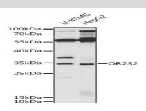
Western blot analysis of extracts of various cell lines, using OR2S2 antibody at 1:1000 dilution.<br/>Secondary antibody: HRP Goat Anti-Rabbit IgG at 1:10000 dilution.<br/>br/>Lysates/proteins: 25ug per lane.<br/>br/>Blocking buffer: 3% nonfat dry milk in TBST.<br/>Detection: ECL Basic Kit .<br/>br/>Exposure time: 10s.
