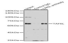
Immunoprecipitation analysis of 300ug extracts of HeLa cells using 3ug TAF6L antibody . Western blot was performed from the immunoprecipitate using TAF6L antibody at a dilution of 1:1000.
