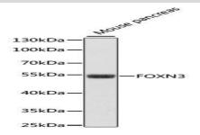
Western blot analysis of extracts of mouse pancreas, using FOXN3 antibody at 1:1000 dilution.<br/>br/>Secondary antibody: HRP Goat Anti-Rabbit IgG at 1:10000 dilution.<br/>br/>Lysates/proteins: 25ug per lane.<br/>br/>Blocking buffer: 3% nonfat dry milk in TBST.<br/>br/>Detection: ECL Basic Kit .<br/>br/>Exposure time: 90s.
