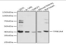
Western blot analysis of extracts of various cell lines, using TFB1M antibody at 1:1000 dilution.<br/>Secondary antibody: HRP Goat Anti-Rabbit IgG at 1:10000 dilution.<br/>br/>Lysates/proteins: 25ug per lane.<br/>br/>Blocking buffer: 3% nonfat dry milk in TBST.<br/>Detection: ECL Basic Kit.<br/>br/>Exposure time: 5s.
